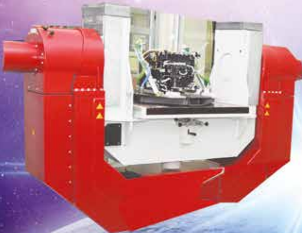
NIUSAT FM on ANGULAR MOTION SIMULATOR (AMS) For HARDWARE IN LOOP (HILS) SIMULATION TEST
